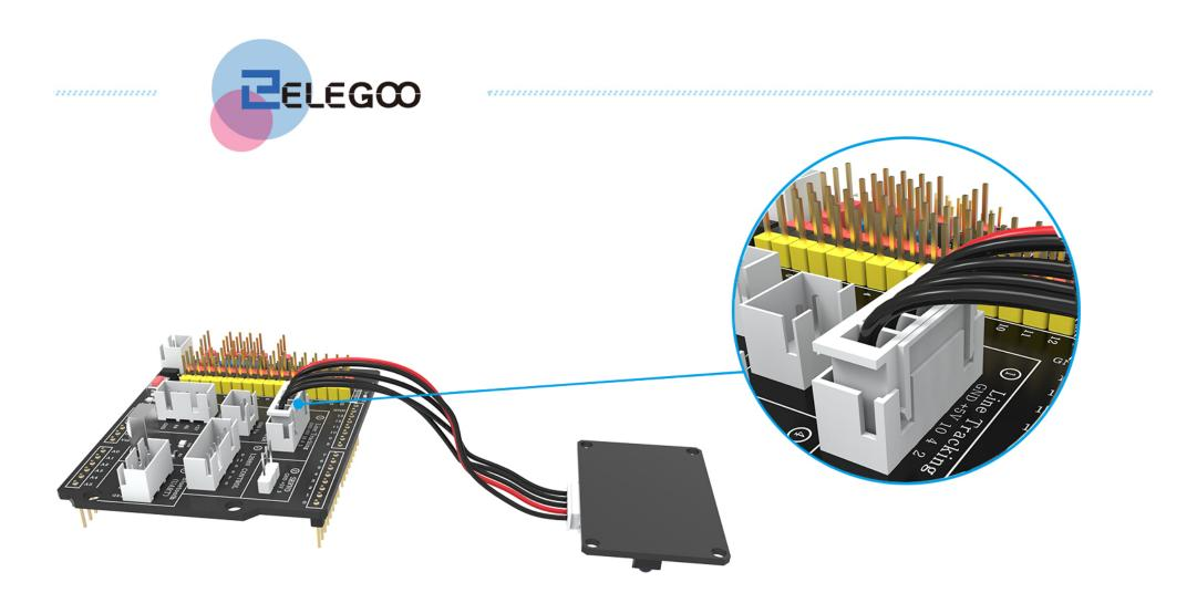
Connect the line tracking module to the expansion board.
