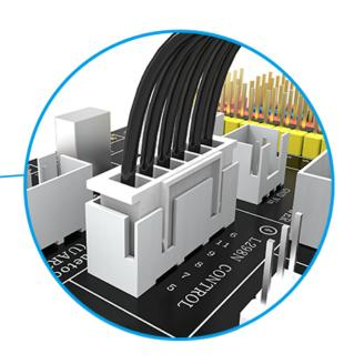
Connect the L298N to the expansion board.
