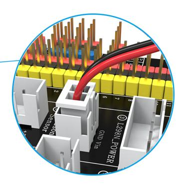
Connect the L298N to the expansion board.
