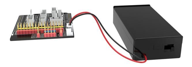
Connect the battery compartment to the expansion board.
