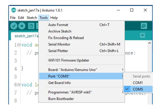
STEP7: Open the file AUTO\_GO\_\AUTO\_GO\_.ino and upload to the UNO controller board
