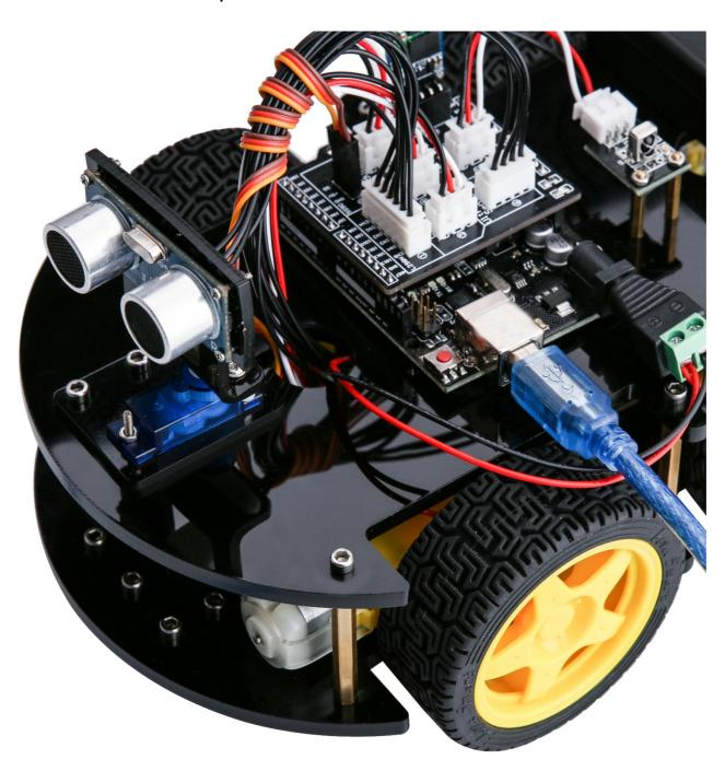
Upload the program to the UNO board, disconnect it from the computer, and then switch on the car's power supply. (TIPS: The bluetooth module should be pulled out when you upload the program every time, or it will be failed to upload the program.)
